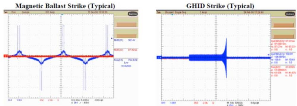
The ineffective and unnecessary re-striking of magnetic ballasts (as shown above in Figure 1.1) greatly deteriorates the electrodes. Evidence of this additional abuse is shown in Figure 1.2 below. Each of these electrodes have driven lamps for 4,000 hours in a 12 hours on and 12 hours off sequence to emulate typical dusk until dawn operation.
